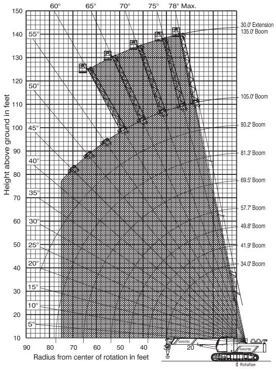
Limits of operation: Maximum load capacity = 750 lb Maximum radius when mounted on main boom = 75 ft
