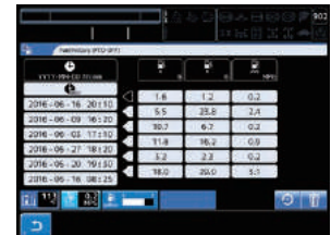
Fuel consumption history display (during traveling)
