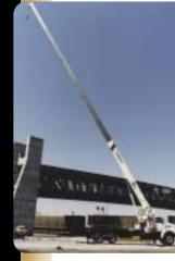
• 33-ton (29.94-t) maximum capacity • 167ft (50.91-m) maximun vertical reach
